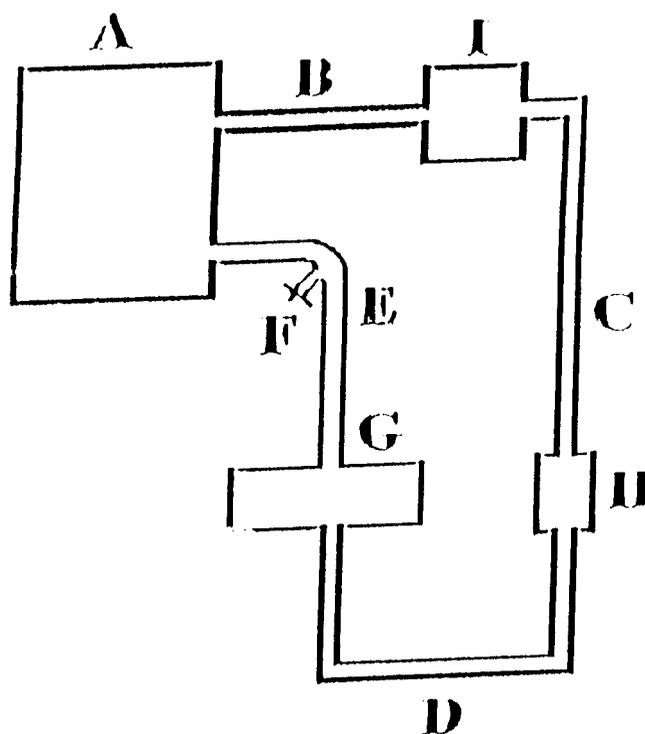
**Figure 1** | Schematic diagram of the laboratory-scale unit. (A) Sterile drum, (B), (C), (D), (E) latex tubing, (F) tap facilitating for sampling, (G) Pedersen device, (H) flow-through glass tube and (I) peristaltic pump.
