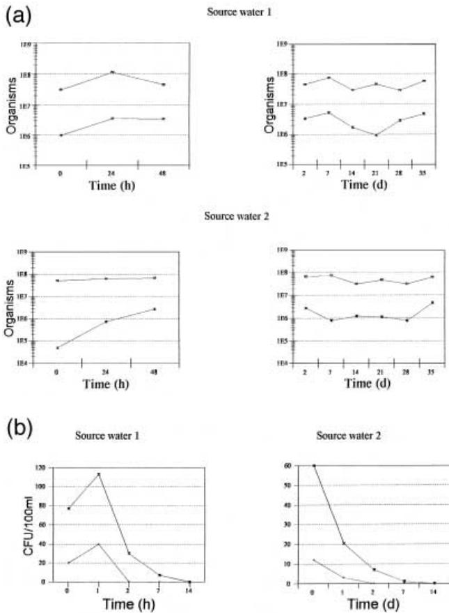
**Figure 2** | (a) Number of total bacteria (TB—epifluorescence) and heterotrophic plate count (HPC) bacteria in the raw water —x— HPC (CFU/ml), —□— TB (cell/ml); (b) recovery of coliform bacteria in the raw water during the experimental period. —x— total coliform, —■— fecal coliform.
