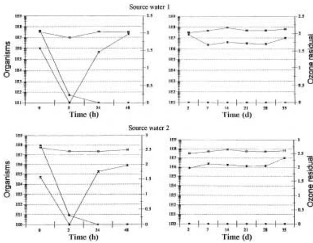
**Figure 5** | Number of total bacteria (TB—epifluorescence) and heterotrophic plate count (HPC) bacteria in the ozonated water —x— HPC (CFU/ml), —□— TB (cell/ml), —◇— ozone residual.
