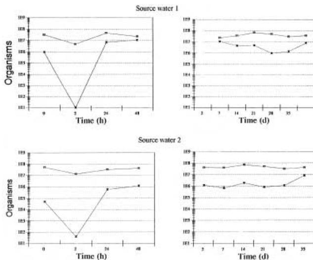
**Figure 6** | Number of total bacteria (TB—epifluorescence) and heterotrophic plate count (HPC) bacteria in the UV irradiated water —x— HPC (CFU/ml), —□— TB (cell/ml).
