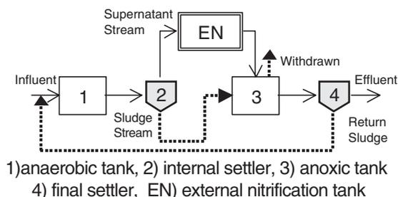
**Figure 1** Configuration of A2N system
