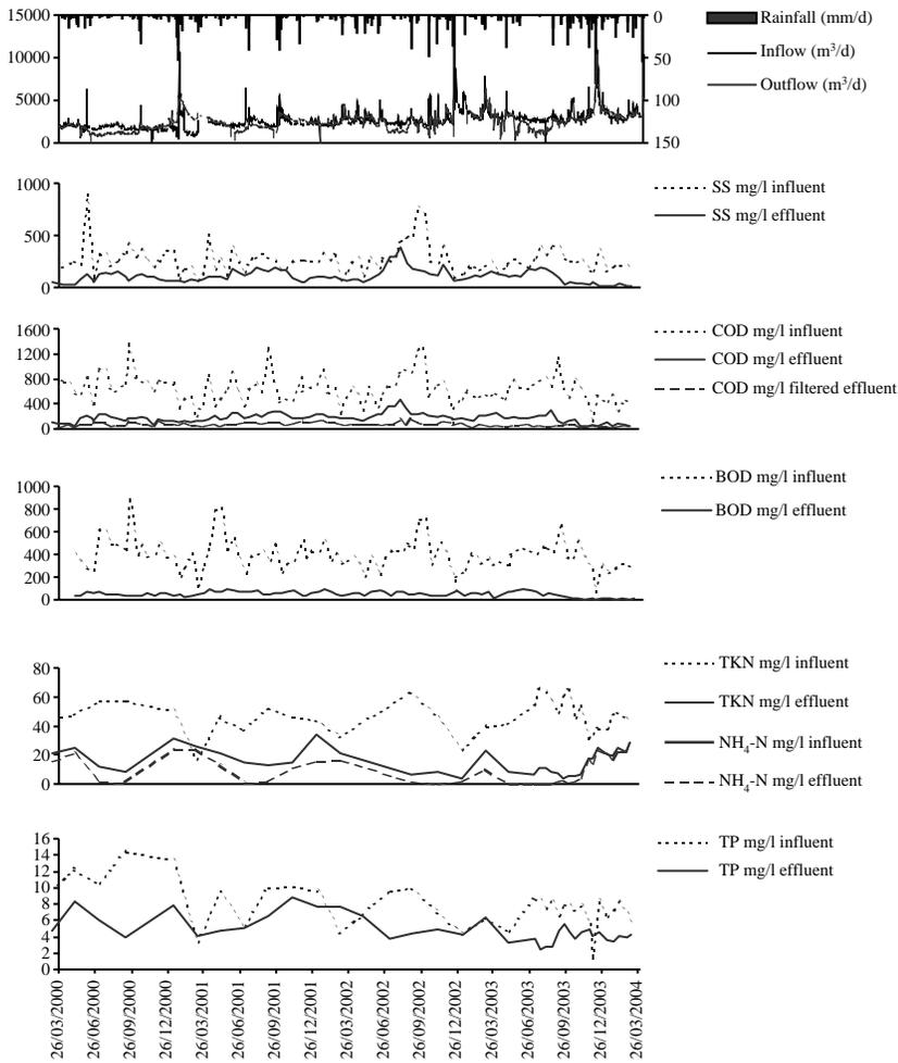
**Figure 2** Times series (2000–2004) of influent wastewater and effluent from Mèze WSP for flow, SS, COD, BOD, Kjeldahl nitrogen (TKN), ammonia (NH<sub>4</sub>-N) and total-P
