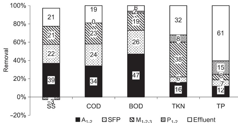
Figure 3 Contribution of each stage of treatment in the overall removal
