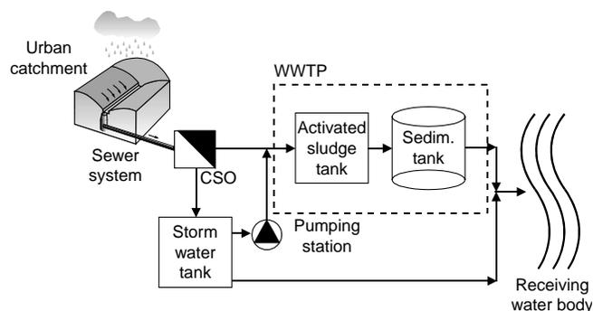
Figure 1 | Schematic representation of the integrated urban drainage system.
