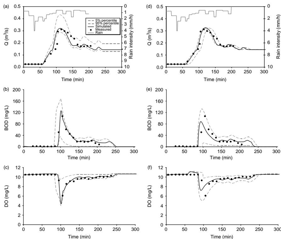
**Figure 5** | Uncertainty bands in terms of flow rate, BOD, and DO for the detailed model [(a), (b), (c)] and for the simplified model approach [(d), (e), (f)].
