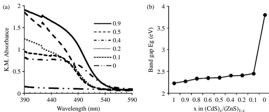
**Figure 4** | Light absorption properties of the catalysts  $(\text{CdS})_x/(\text{ZnS})_{1-x}$ .
