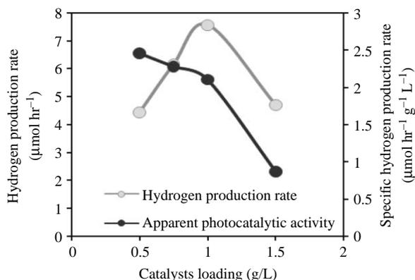
**Figure 6** | The effect of the catalyst load on photocatalytic hydrogen generation by  $(\text{CdS})_{0.9}/(\text{ZnS})_{0.1}$  under visible light (165W Xe lamp) in 60 ml solution containing 0.2 M  $\text{Na}_2\text{SO}_3$  and 0.1 M  $\text{Na}_2\text{S}$ .
