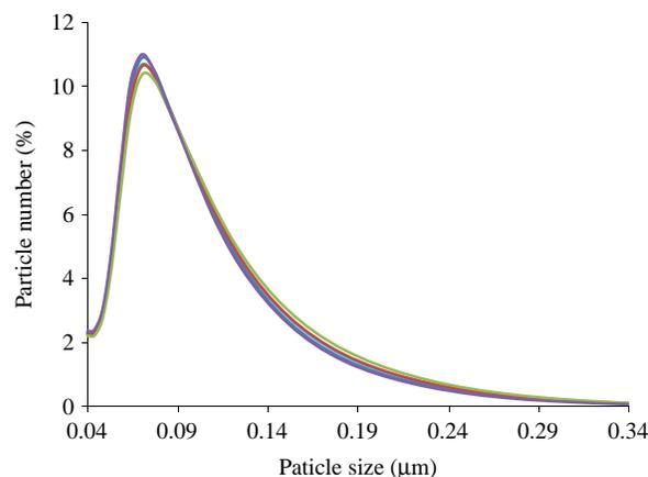
Figure 1 | Particle size distribution of the catalysts.
