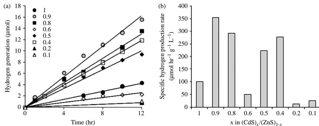
**Figure 5** | Photocatalytic  $\text{H}_2$  generation with different catalysts  $(\text{CdS})_x/(\text{ZnS})_{1-x}$  under visible light (100W Hg lamp), 1 g/L catalyst in 60 ml solution containing 0.2 M  $\text{Na}_2\text{SO}_3$  and 0.1 M  $\text{Na}_2\text{S}$ .
