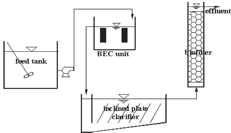
**Figure 2** Schematic of BEC/biofiltration system for continuous flow test
