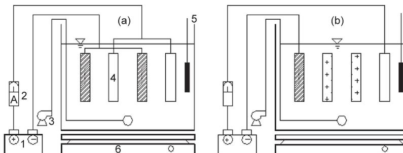
**Figure 1** Schematic of electrocoagulation reactors. Monopolar electrocoagulation unit (a) and Bipolar electrocoagulation unit (b). 1: DC power supply, 2: Digital multimeter, 3: Aerator, 4: Electrodes, 5: DO and pH meter, 6: Stirrer
