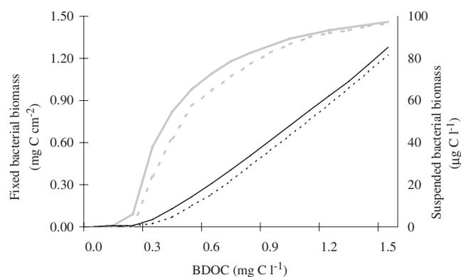
**Figure 4** | Evolution, as a function of the BDOC concentration in the discharged water, of the maximum fixed (grey lines) and free (black lines) bacterial biomass reached in the system. The dotted lines represent the values obtained with a free chlorine residual at the plant outlet of 1 mg Cl<sub>2</sub> l<sup>-1</sup> and the solid lines represent the values obtained with no chlorine residual.
