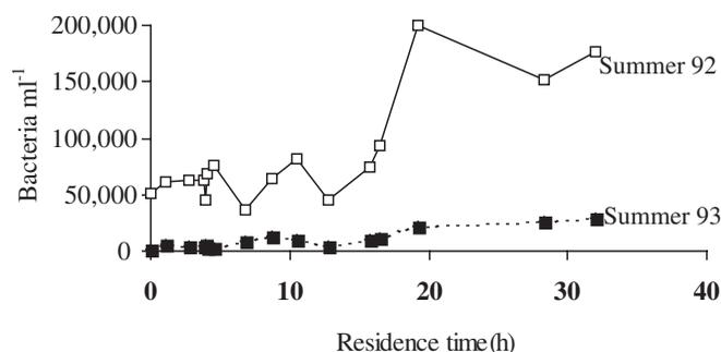
**Figure 3** | Bacteria counts by epifluorescence microscopy in Auvers-sur-Oise distribution system (northern Parisian suburbs) plotted against residence time, before (summer 1992) and after (summer 1993) feeding with nanofiltered water (after Randon *et al.* 1995; Laurent *et al.* 1999).
