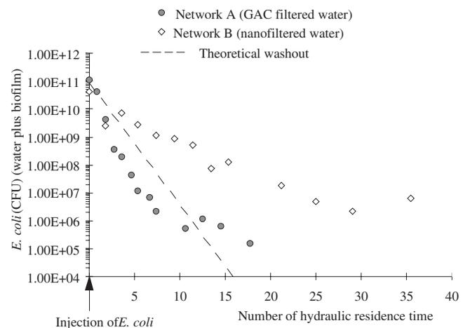
**Figure 2** | Density of *E. coli* (CFU) (water plus biofilm) in the first loop of network A supplied with GAC water (hydraulic residence time=24 h per loop) and network B supplied with nanofiltered water (hydraulic residence time=12 h per loop). Without chlorine residual (after Sibille *et al.* 1998).
