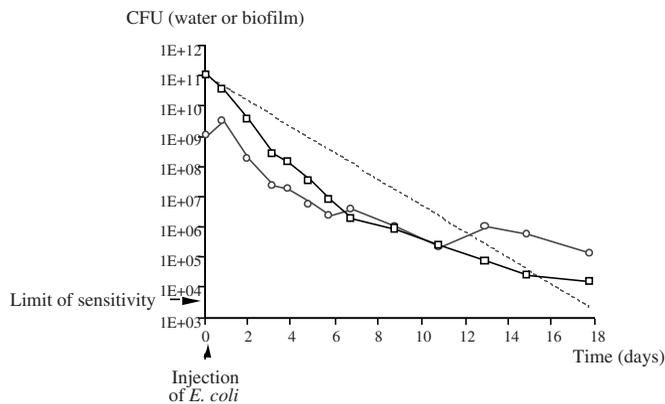
**Figure 1** | Behaviour of *Escherichia coli* experimentally introduced into the distribution system (squares, water; circles, biofilm; dotted line, theoretical washout) in the absence of chlorine residual (after FASS *et al.* 1996).
