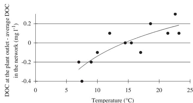
**Figure 6** | DOC consumption in the network, as a function of water temperature ( $y = -0.38 \ln(X) - 1.02$ ,  $r^2 = 0.70$ ).
