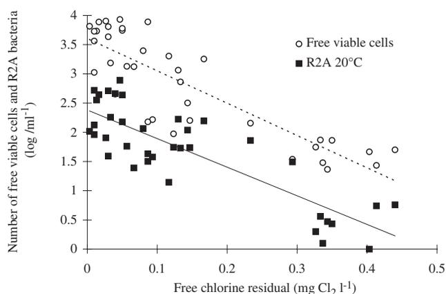
**Figure 5** | Number of bacteria as a function of free chlorine residual concentration in the Parisian suburbs distribution system. The dotted line represents the linear regression for the respiring (CTC+) bacterial cells ( $y = -5.56 X + 3.61$ ,  $r^2 = 0.74$ ) the plain line represents the linear regression for the R2A counts cells ( $y = -4.89 X + 2.38$ ,  $r^2 = 0.70$ ).
