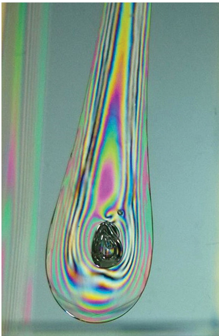
FIG. 3. Isochromatics through PRD1 obtained using white light. In the center of the head of the PRD 1 (head diameter 7.4 mm) is a vacuole and the colour fringes exist throughout the PRD. Fringes exist very close to the vacuole, indicating the existence of residual stresses in all parts of the drop.
