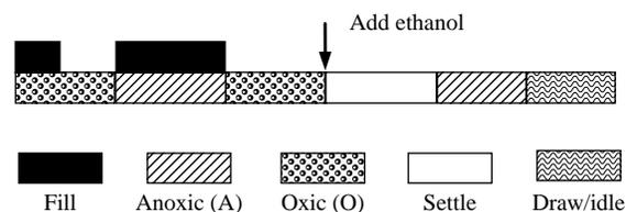
Figure 2 | Operation strategy in step-feed CAST.
