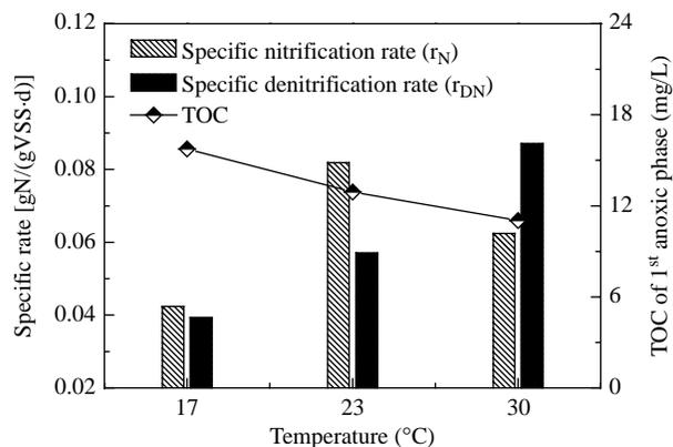
**Figure 5** | Effect of temperature on both nitrification and denitrification in step-feed CAST with real time control.
