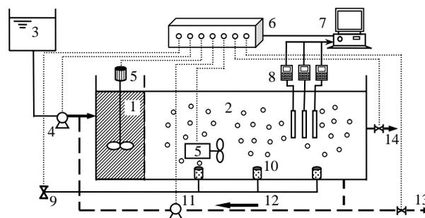
**Figure 1** | Schematic diagram of experimental system and control equipment in CAST. 1. selector 2. complete mix zone 3. influent tank 4. influent pump 5. mixer 6. real-time control system 7. computer 8. DO, ORP, pH sensors 9. air pump 10. air diffuser 11. returned activated sludge pump 12. return activated sludge 13. excess sludge 14. effluent.
