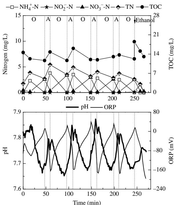
**Figure 6** | Profiles of  $\text{NH}_4^+\text{-N}$ ,  $\text{NO}_2^-\text{-N}$ ,  $\text{NO}_3^-\text{-N}$ , TN, TOC and pH, ORP with high C/N influent during one typical cycle.
