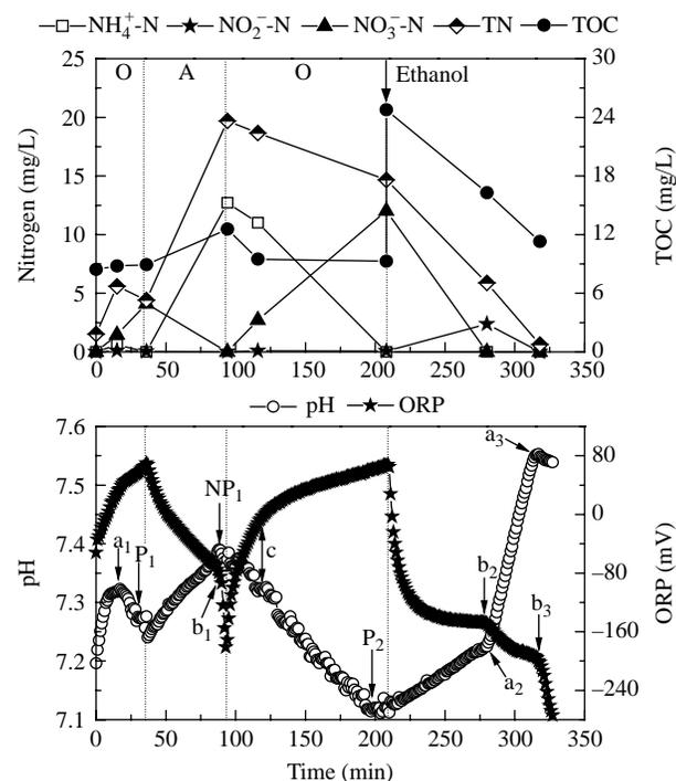
**Figure 3** | Profiles of  $\text{NH}_4^+\text{-N}$ ,  $\text{NO}_2^-\text{-N}$ ,  $\text{NO}_3^-\text{-N}$ , TN, TOC and pH, ORP during a typical cycle.
