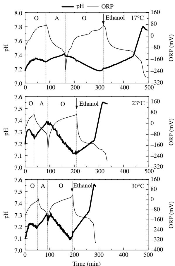
**Figure 4** | Experimental pH and ORP profiles under different temperature.
