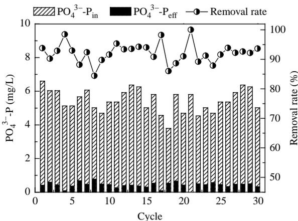
**Figure 7** | Performance of phosphorus removal in step-feed CAST with real time control.
