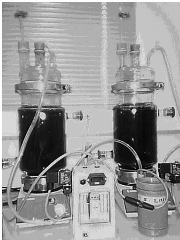
**Figure 1** Picture of the reactor used for BMP assays
