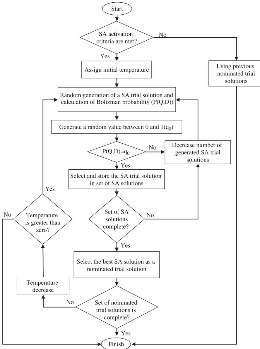
Figure 2 | Simulated annealing flowchart (Bozorg Haddad et al. 2007).
