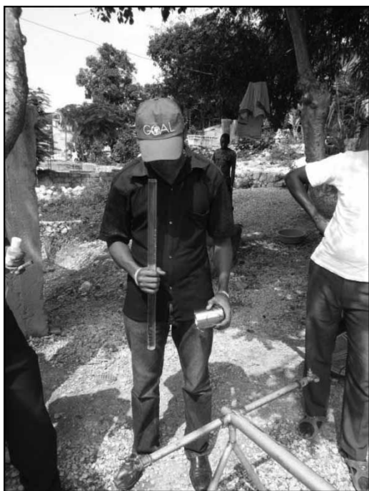
Figure 1 | Turbidity field measurement with a turbidity tube.
