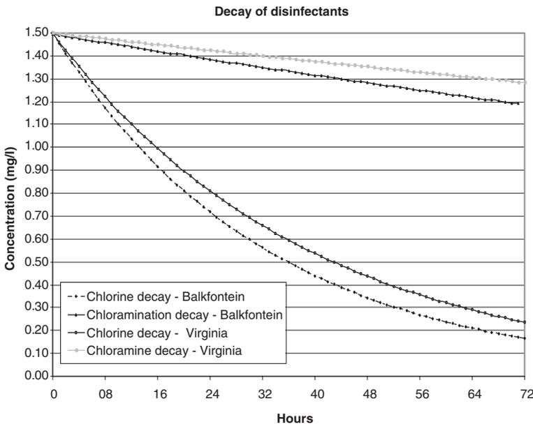
**Figure 1** Decay of chlorine and monochloramine
