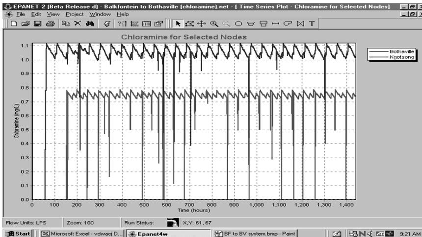
**Figure 4** Monochloramine levels in the reservoirs of Bothaville and Kgotsong
