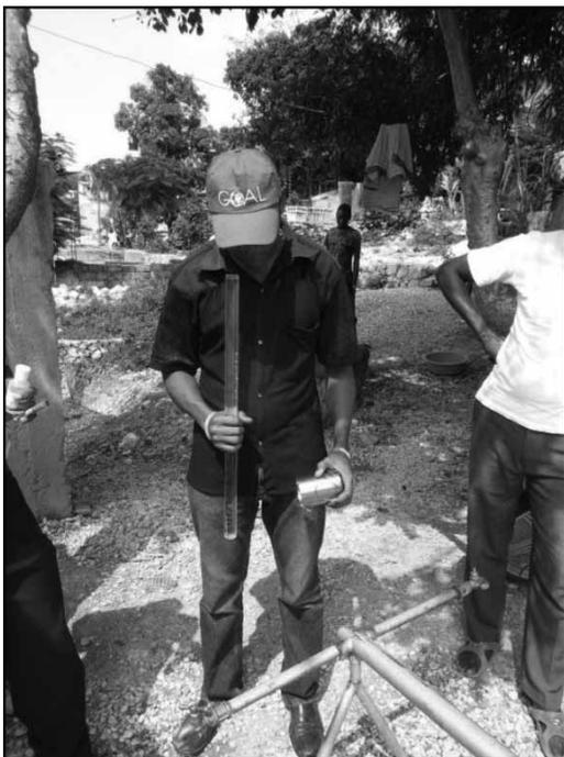
Figure 1 | Turbidity field measurement with a turbidity tube.
