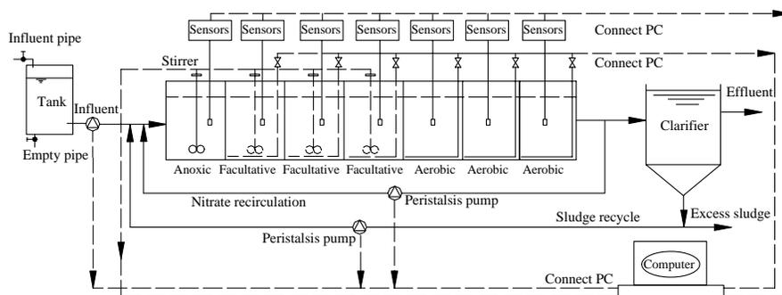
Figure 1 A schematic view of the bench-scale reactor system
