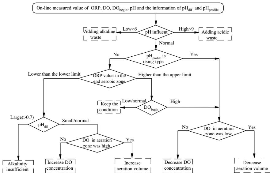
**Figure 8** The inference procedure of the proposed fuzzy logic controller
