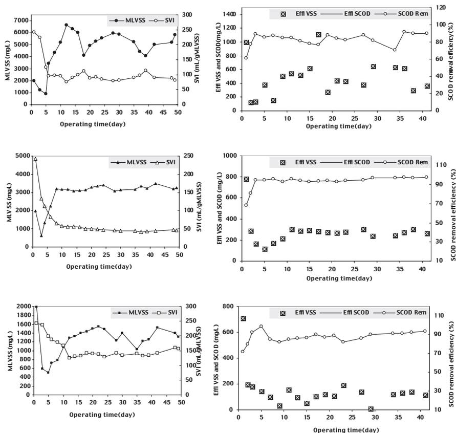
**Figure 1** Reactor performance under different OLR. Top, middle and bottom, the applied OLR are 8, 4 and 2 kg COD·(m<sup>3</sup>·d)<sup>-1</sup> respectively
