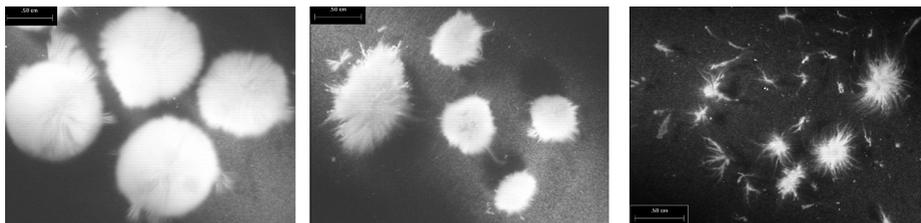
**Figure 2** Stereomicroscopic pictures of aerobic granules. From A to C, the applied OLR are 8, 4 and 1 kg COD ·(m<sup>3</sup>·d)<sup>-1</sup> respectively
