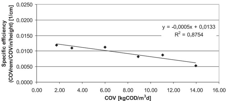
**Figure 3** Specific removal efficiencies of BAF with plastic media
