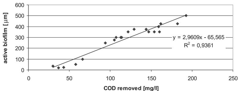
**Figure 4** Active biofilm thickness versus removed COD of BAF with plastic media
