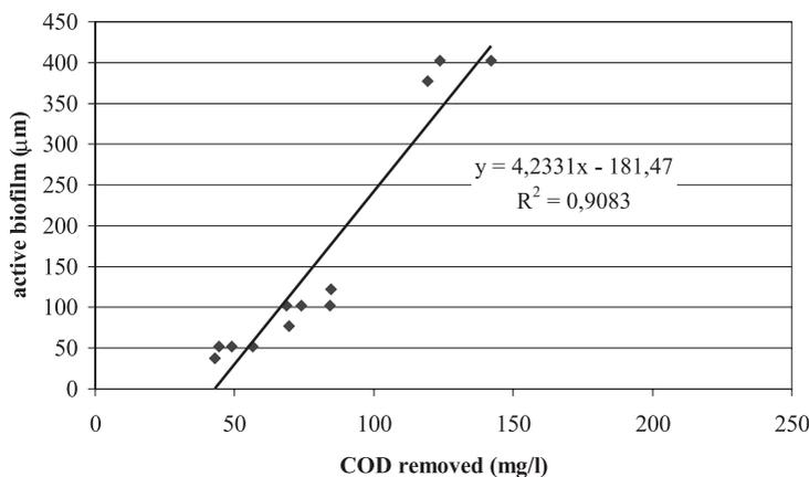
**Figure 8** Active biofilm thickness versus removed COD of BAF with Arlita media
