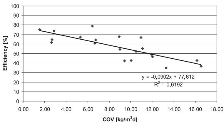
**Figure 2** COD removal efficiency of BAF with plastic media
