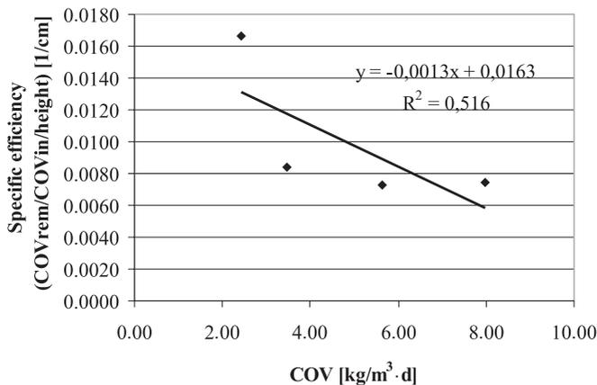
**Figure 7** Average specific removal efficiency of BAF with Arlita media
