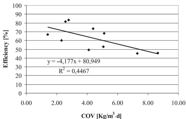
**Figure 6** COD removal efficiency of BAF with Arlita media
