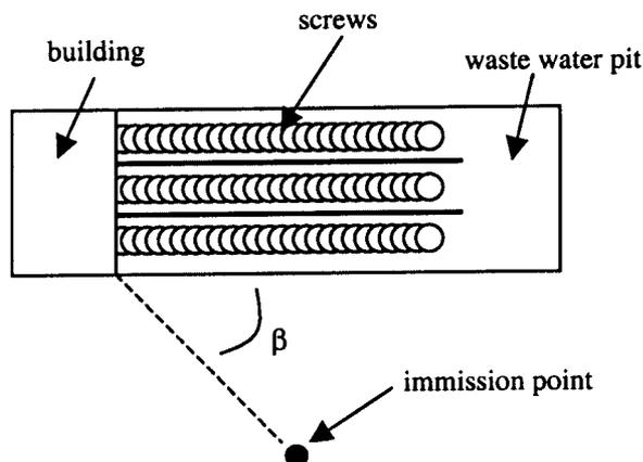
**Figure 4** Top view of a screw pump configuration with definition of the angle  $\beta$  for calculation of the directivity index DI (Table 1) (VROM, 1981)
