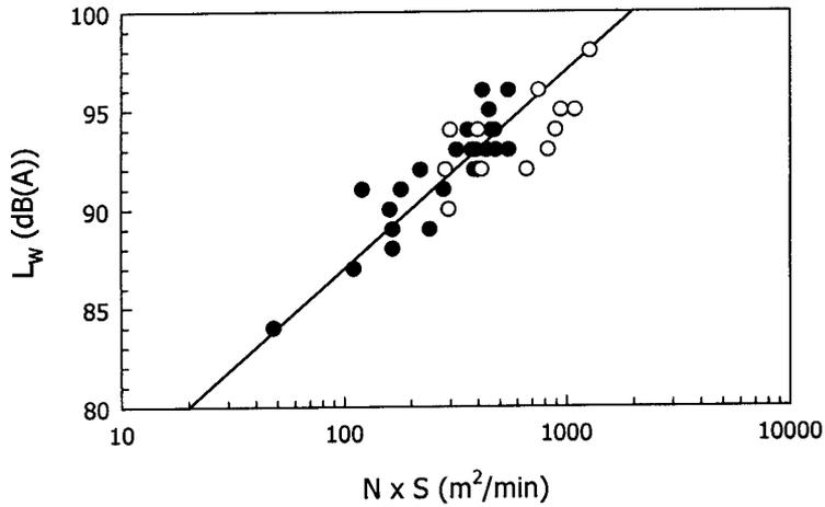
**Figure 5** The sound power level ( $L_w$ ) of the splashing water of a screw pump (—) (Equation 3) in comparison to the (corrected) historical data owned by Peutz & Associés (●) and the field data measured at the Aquafin WWTP's (O)
