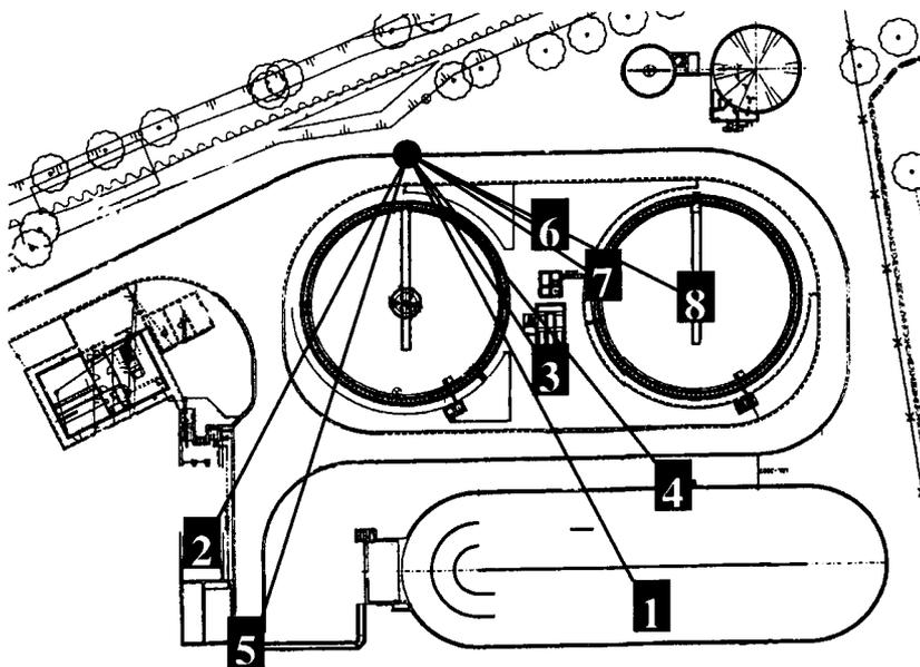
**Figure 6** Lay-out of the WWTP of Landen with location of the immersion point (●) and the different sound sources and considered in Table 2: (1) aerator, (2) screw pump, (3) screw pump, (4) overflow weir, (5) overflow weir, (6) overflow weir and (7) overflow weir
