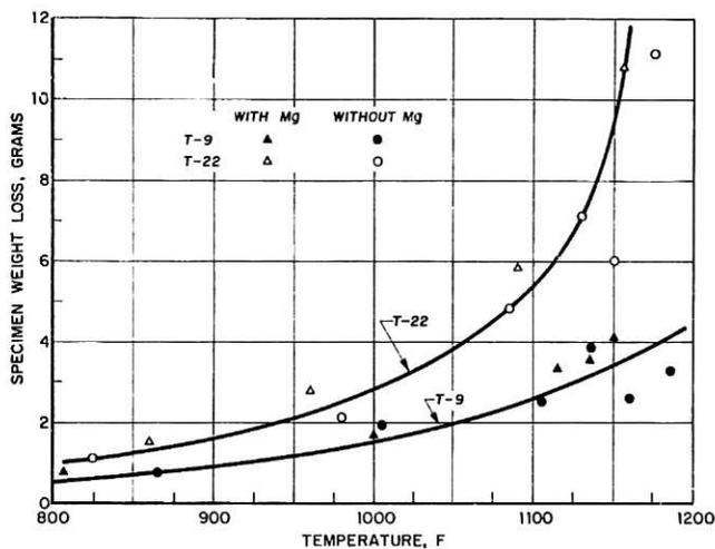
Fig. 15 Oil-ash corrosion of ferritic alloys as a function of temperature
