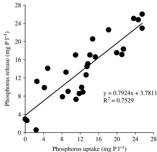
**Figure 9** Phosphorus release versus phosphorus uptake profile of the activated sludge of AU8 of Jurong WRP (26 April–11 August 2005)
