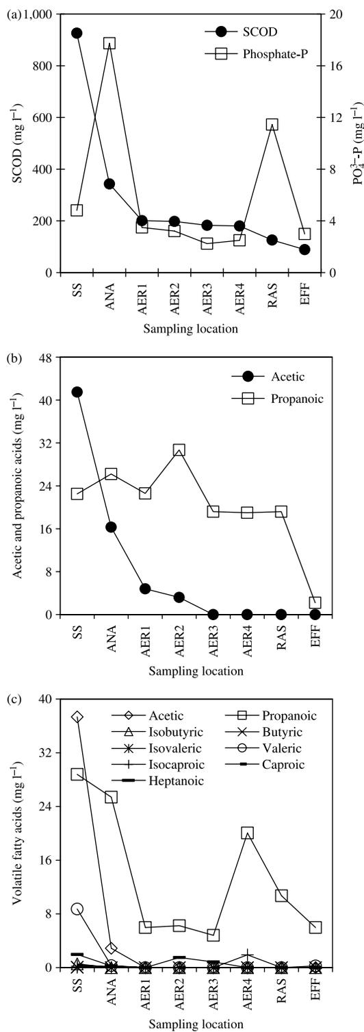
**Figure 6** (a) SCOD and  $PO_4^{3-}$ -P concentration profiles at different sampling locations of AU8 of Jurong WRP (20 September 2005); (b) Acetic and propanoic acids concentration profiles at different sampling locations of AU8 of Jurong WRP (20 September 2005); (c) Volatile fatty acids concentration profiles at different sampling locations of AU8 of Jurong WRP (20 September 2005)
