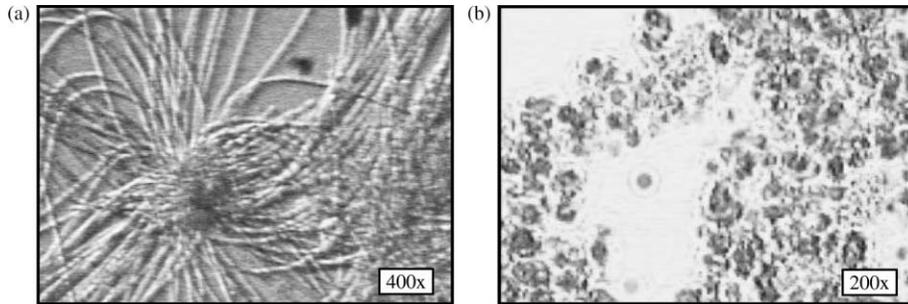
**Figure 4** (a) Microscopic image of the sludge taken from the activated sludge unit of Jurong WRP without anaerobic selector operation (26 June 2005); (b) Microscopic image of the sludge taken from AU8 of Jurong WRP (26 June 2005)
