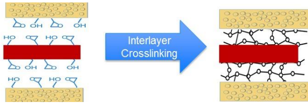
Fig. 9. Interlayer crosslinking between mold epoxy layers and lead frame with hydroxy and epoxy functional groups
