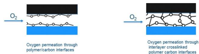
Fig. 8. Oxygen permeation through non-crosslinked cathode layer interfaces and interlayer crosslinked cathode interfaces.
