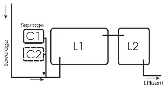
**Figure 1** Alcorta (Argentina) pond scheme. C1 + C2 = alternately-operated septage sedimentation/digestion ponds; L1 + L2 = facultative and maturation ponds co-treating septage supernatant and raw wastewater
