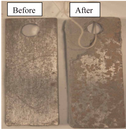
Figure 5 | Comparison of the ductile iron coupons with and without corrosion after testing and the removal of cement lining.
