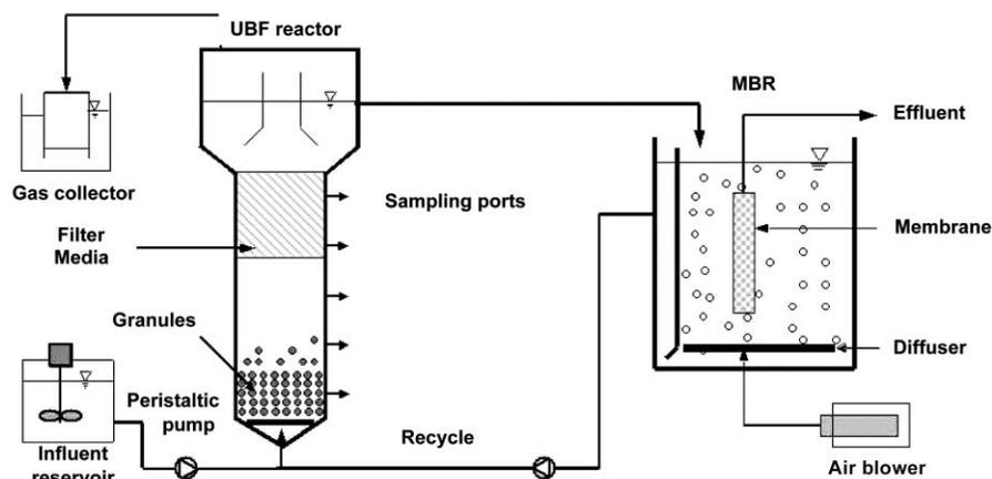
Figure 1 Schematic diagram of the combined UBF/MBR system
