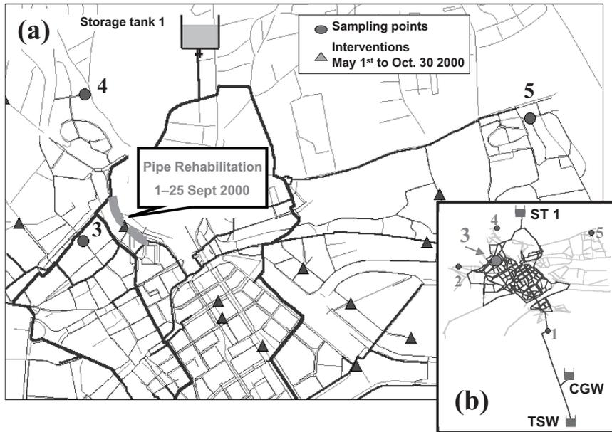
**Figure 4** (a) Results of a time/space query for interventions around sampling points 3, 4, 5 where positive coliform samples were collected on 30 October 2000. (b) All possible upstream hydraulic paths supplying sampling point #3 (derived from Epanet results)
