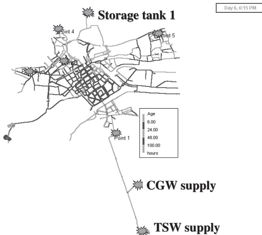
**Figure 1** Hydraulic model of the zone under study and location of the DS supply, storage and sampling points
