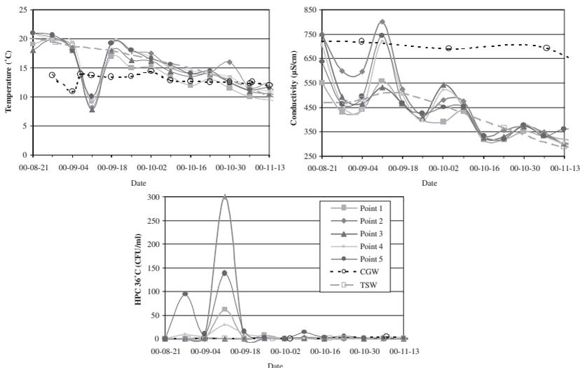
**Figure 3** Weekly monitoring of the water quality parameters at the five sampling points from August–November 2000
