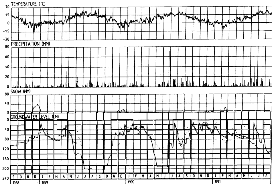
Fig. 11. Simulation of groundwater level for the independent period from September 1988 until August 1991 at Zemnieki (dots – observed levels).
