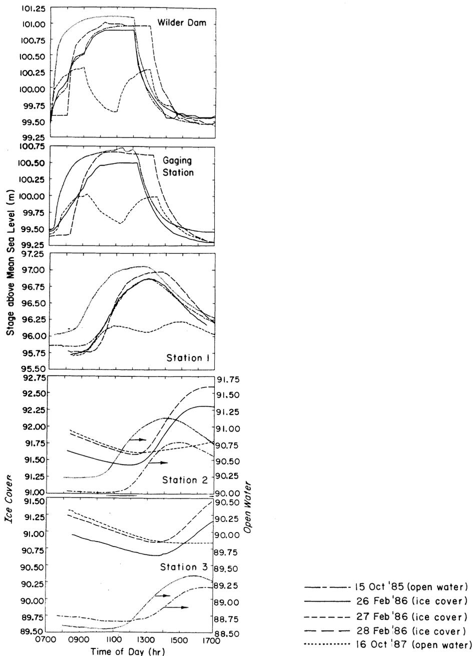
Fig. 2. Measured stage during the fall and winter tests as a function of time at several locations in the study reach. The stage data at stations 2 and 3 required separate vertical scales to present both the ice cover and the open water results.
