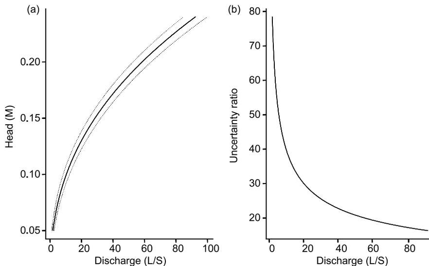
**Figure 5** (a) Head–discharge equation for the thin plate v-notch weir at Sandsli gauging station with 95% confidence limits (dotted lines). (b) Uncertainty ratio plot for the estimated discharges at Sandsli gauging station
