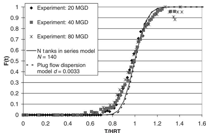
**Figure 7** | Single parameter model predictions of the Marston RTD using contactor  $L/W$  ratio to compute  $N$  and  $d$  values (experimental data sets were normalized with calculated HRT).
