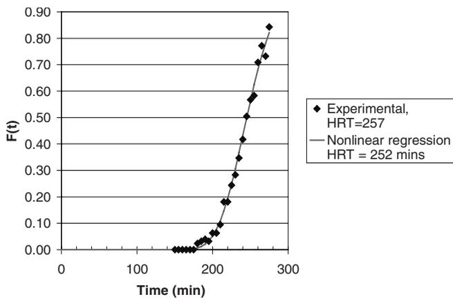
Figure 5 | Nonlinear least squares analysis of experimental tracer tests at 20 MGD.
