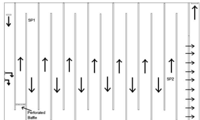
Figure 3 | Schematic of Marston WTP contactor.
