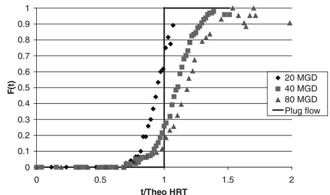
Figure 4 | Experimental RTD function for Marston contactor; time normalized with theoretical HRT.
