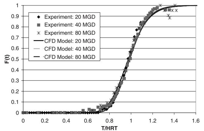
Figure 6 | Comparison between numerical and experimental RTD curves (experimental data sets were normalized with calculated HRT).
