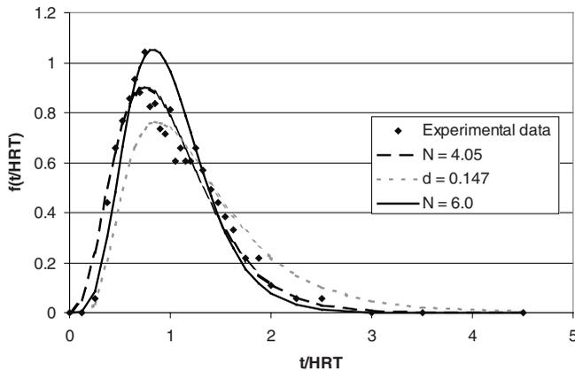
**Figure 1** | Comparison between experimental and direct numerical model residence time density curves: complete mix tanks in series model ( $N$ ) and PFD model ( $d$ ).
