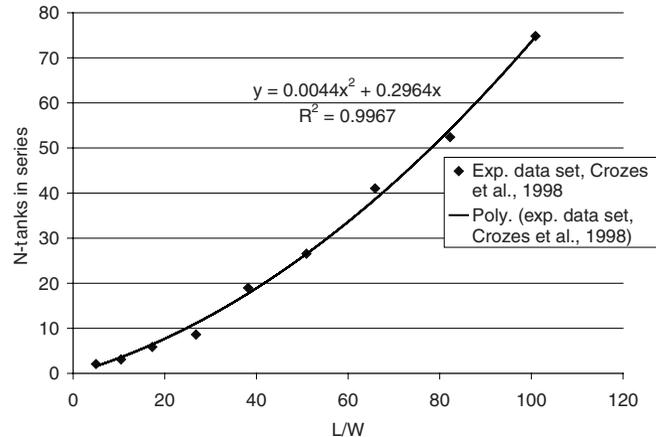
**Figure 2** | Data conversion for reactor length to width ratio to  $N$  for  $N$ -tanks in series model.
