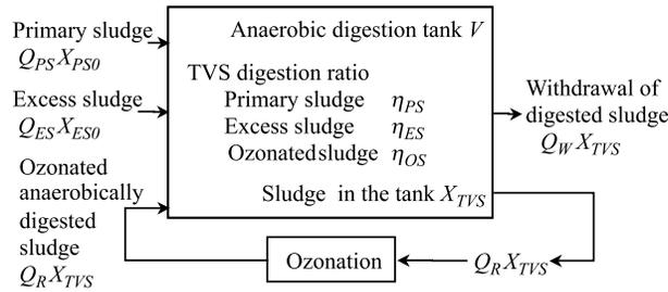
**Figure 7** Illustration of TVS digestion by the high-concentrated AD process with partial ozonation
