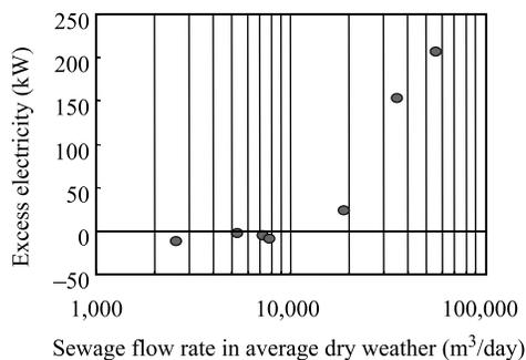
**Figure 9** Energy recovery with power generation \* Electricity generation efficiency ( $\text{kJ-electricity produced}/\text{kJ-methane}$ ) = 26%: below 10,000  $\text{m}^3$ -sewage/day, 30%: 10,000–20,000  $\text{m}^3/\text{day}$ , 37%: beyond 20,000  $\text{m}^3/\text{day}$
