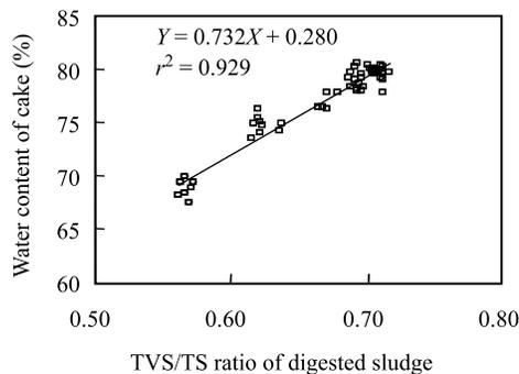
Figure 6 Reduction of cake volume by lowering TVS/TS ratio of sludge
