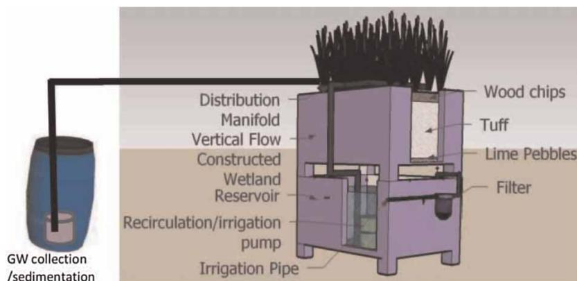
**Figure 1** | Schematic of the on-site RVFCW GW treatment system (after *Alfiya et al. 2013*).
