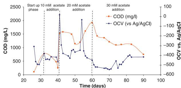
Figure 4 | Influence of increasing acetate concentration on OCV of carbon cloth anode half cell. The dotted lines indicate the addition of acetate (10 mM acetate corresponds to 700 mg/L COD).
