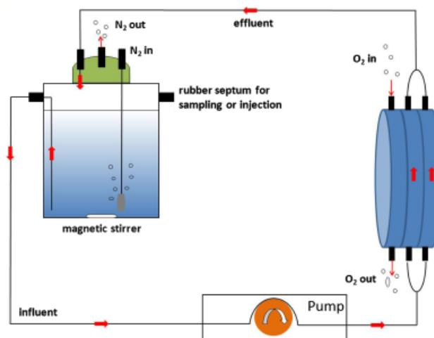
Figure 1 | Schematic drawing of the MFC half cell in recycled batch flow mode.
