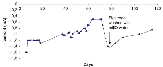
**Figure 7** | Current production by 0 wt% Pt AC cathode poised at  $-100$  mV vs Ag/AgCl.
