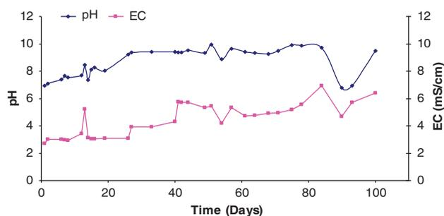
Figure 2 | pH and EC in carbon cloth anode half cell.
