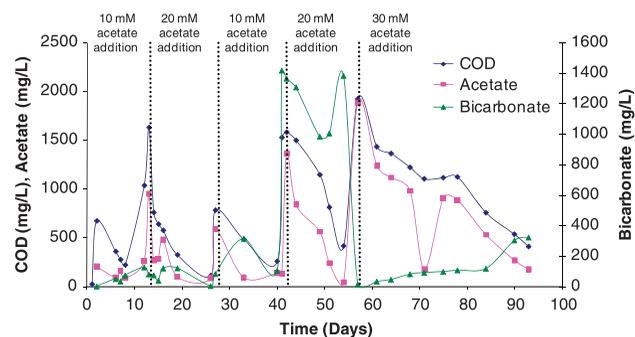
Figure 3 | COD, acetate and bicarbonate carbon cloth anode half cell. The dotted lines indicate the addition of acetate (10 mM acetate corresponds to 700 mg/L COD).
