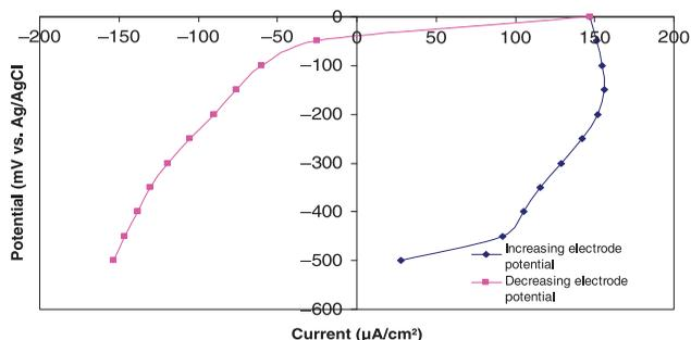
**Figure 6** | Polarization curve of expanded graphite cloth anode half cell.
