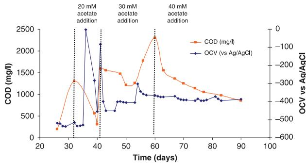
**Figure 5** | Influence of increasing acetate concentration on OCV of expanded graphite cloth anode half cell. The dotted lines indicate the addition of acetate (10 mM acetate corresponds to 700 mg/L COD).
