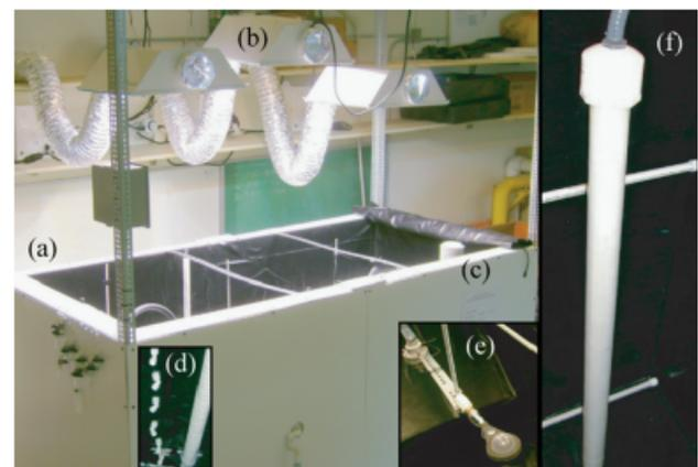
**Figure 2** | (a) Experimental solar pond; (b) high-intensity discharge lamps; (c) air temperature and relative humidity sensor; (d) manual sampling system; (e) net radiometer and pyranometers; (f) vertical high-resolution DTS pole.
