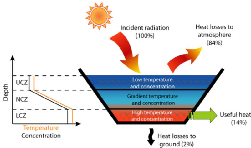
**Figure 1** | Schematic of a salt-gradient solar pond; modified from Kurt *et al.* (2000).
