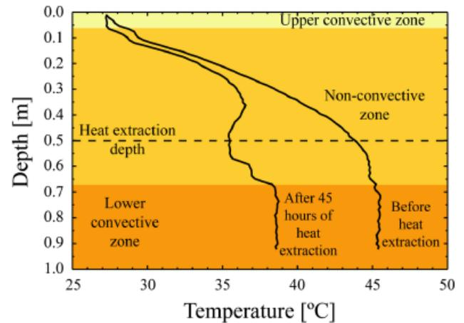
**Figure 5** | Temperature profile inside the solar pond at the beginning and at the end of a heat extraction experiment.
