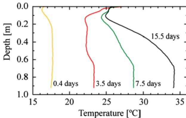
**Figure 4** | Thermal profile for different times during the experiment.
