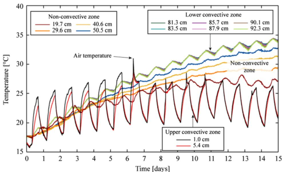
Figure 3 | Thermal evolution at different depths inside the solar pond.
