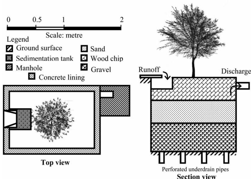
Figure 1 | Schematic diagram of the tree box filter.
