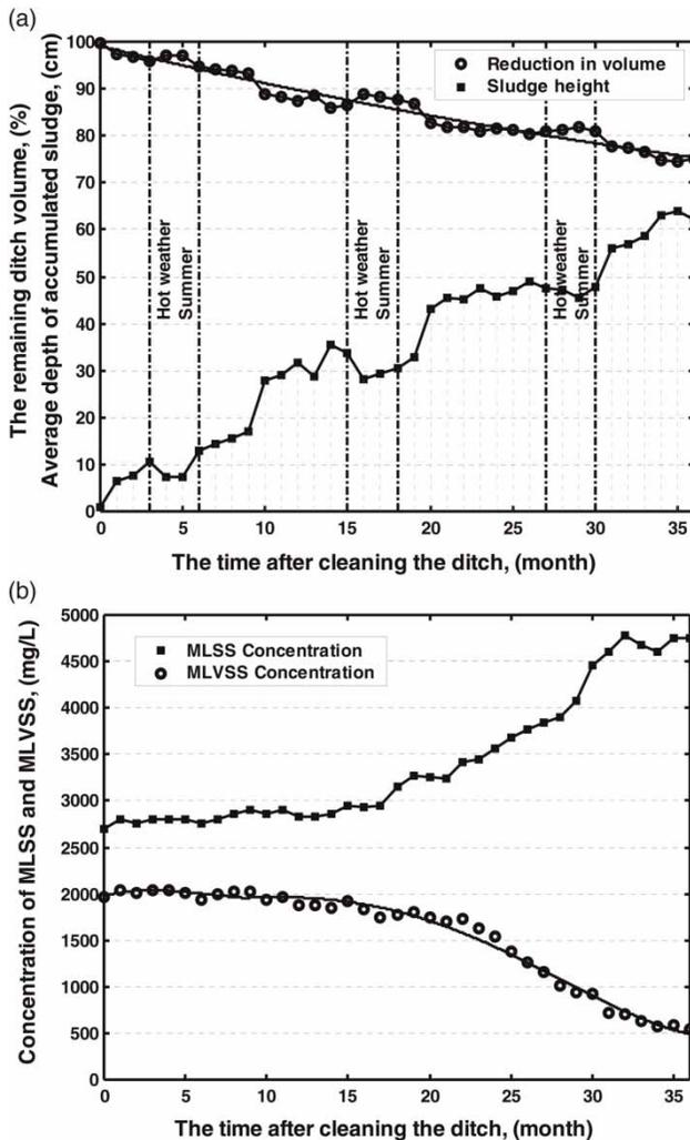
**Figure 3** | (a) Accumulated sludge and volume reduction against operation time after cleaning the ditch. (b) Concentration of MLSS and MLVSS against operation time after cleaning the ditch.
