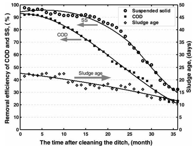
**Figure 4** | Removal efficiency of COD and SS as well as sludge age against operation time after cleaning the ditch.
