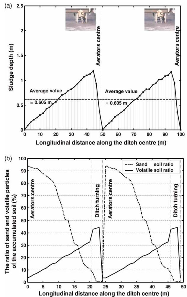
**Figure 2** | (a) Profile of sludge depth along the ditch. (b) Ratio of sand and volatile particles of the accumulated soil along the ditch centre.
