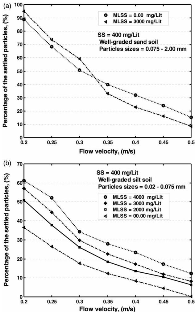
Figure 6 | (a) Settling of sand particles against flow velocity (laboratory verification). (b) Settling of silt particles against flow velocity (laboratory verification).
