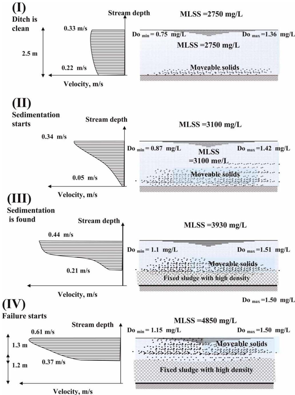
**Figure 5** | Sludge accumulation phases in the OD at the critical sections. I – Ditch is clean, II – Sedimentation starts, III – Sedimentation is found, and IV – Failure starts.
