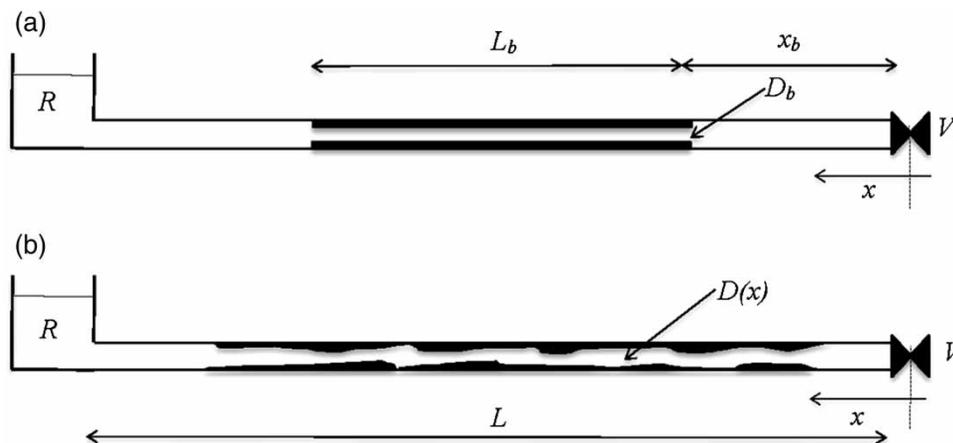
**Figure 2** | Modeling of the extended partial blockage according to (a) Brunone *et al.* (2008a) and Duan *et al.* (2012) and (b) Massari *et al.* (2012). V and R stand for valve and reservoir, respectively.
