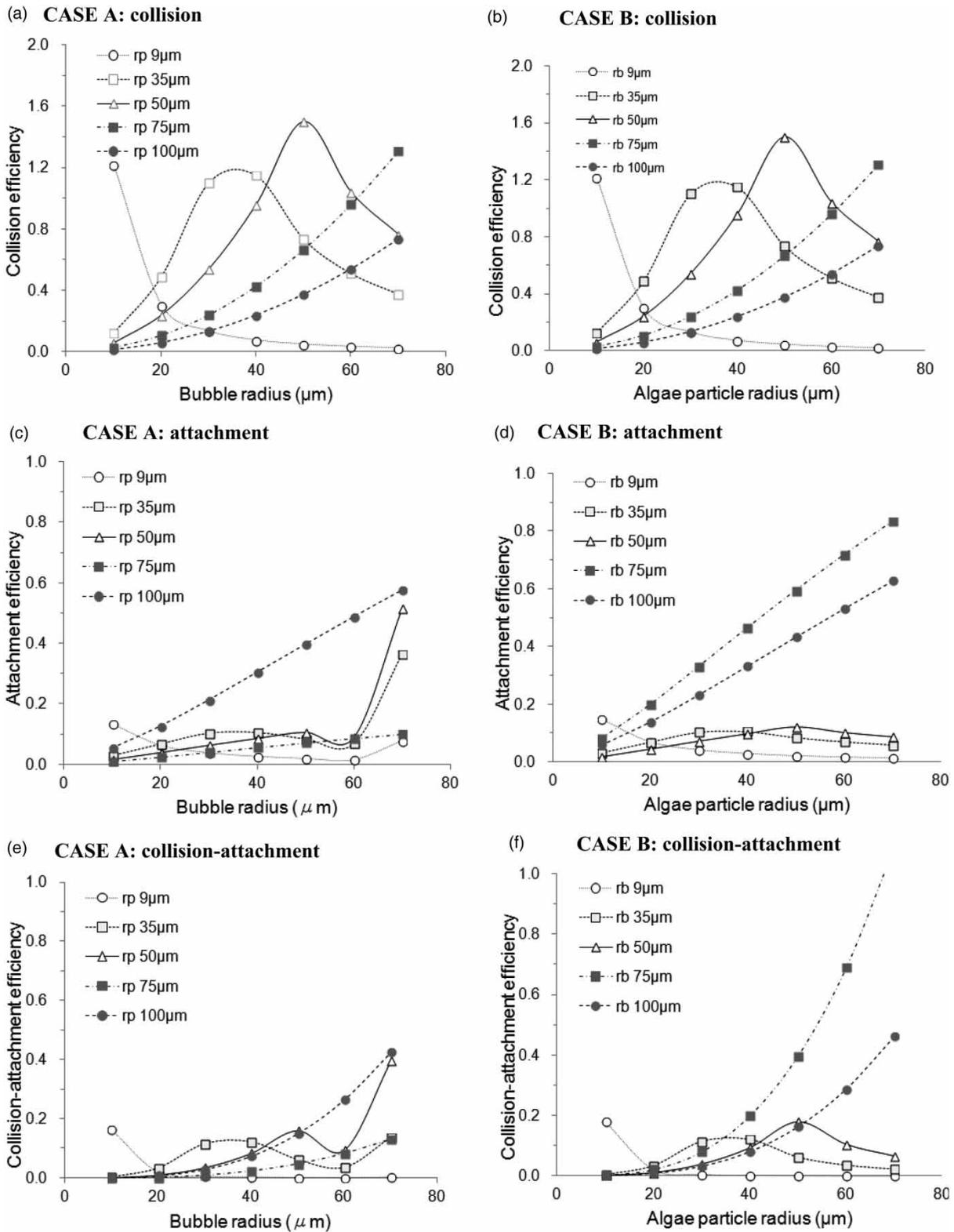
Figure 2 | Size effect on efficiency for Case A and Case B.
