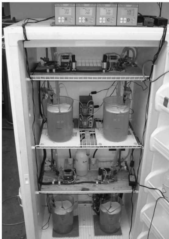
Figure 1 | Laboratory scale SBRs.
