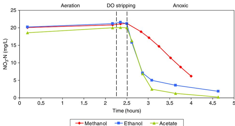
Figure 2 | Example of a typical nitrate profile in an SBR.
