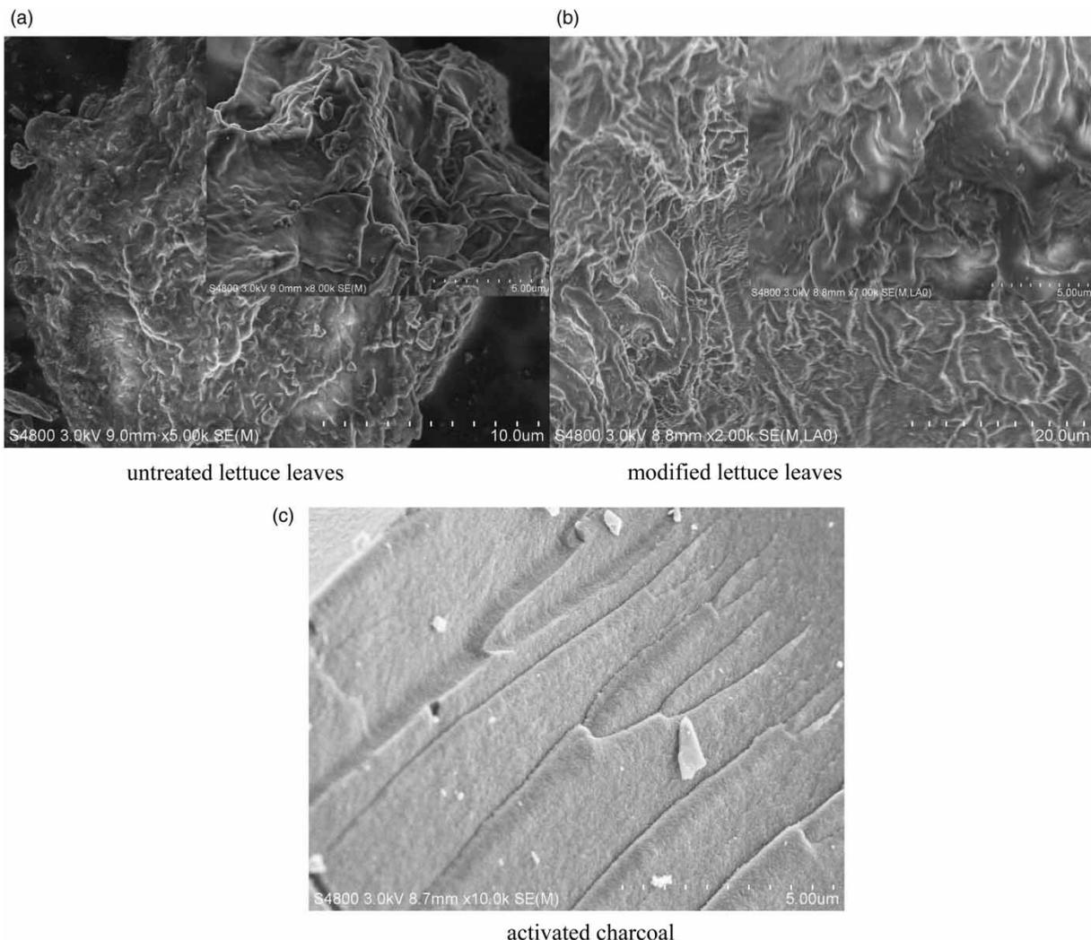
**Figure 5** | The mainly structural changes of lettuce leaf slag after adsorption, and its similar loose structures to activated carbon.
