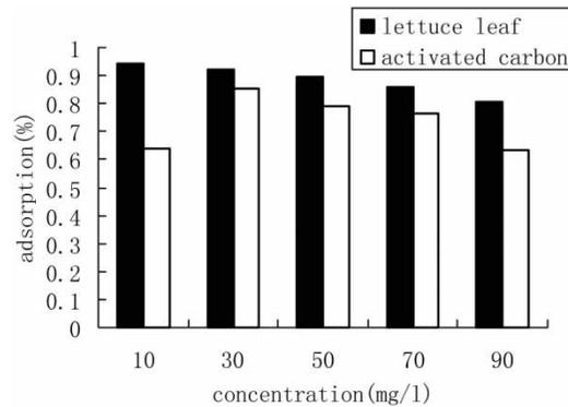
**Figure 2** | Comparing slag with activated carbon, the modified lettuce leaf slag adsorption rate for chromium was better than activated carbon in general. Results represent the means of three independent experiments.
