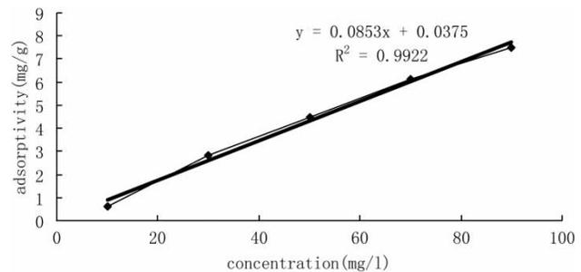
**Figure 3** | The figure shows the relationship between the balance concentration of  $\text{Cr}^{6+}$  and adsorption at 40 °C. The adsorption isotherm is almost straight when the equilibrium concentrations are in the range 40–60 mg/L. Values are averages of three independent experiments.
