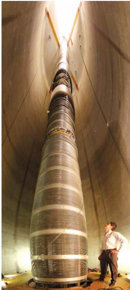
The tandem Van der Graaff accelerator at Australian National University is among the many facilities across Australia for which future funding hangs in the balance. The source of accelerated ions is at the top of the 35-meter-high column.
