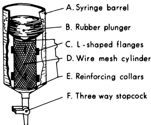
FIG. 1. Digestion-filtration apparatus.
