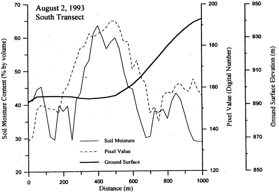
Fig. 3c. Ground surface elevation, SAR pixel value and field measured soil moisture content for the south transect, August 2, 1993.
