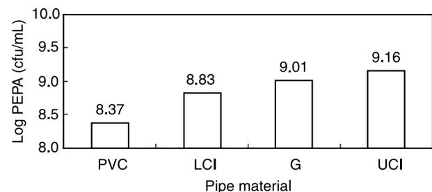
**Figure 7** | Biofilm density (log PEPA) versus pipe material. PVC = Polyvinylchloride, LCI = Lined Cast Iron, UCI = Unlined Cast Iron, G = Galvanized Steel, PEPA = potential exoproteolytic activity.
