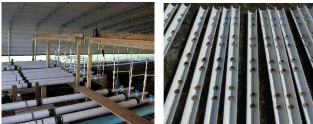
**Figure 2** | Cradles of pilot plant (left) and coupons in the cradles (right).
