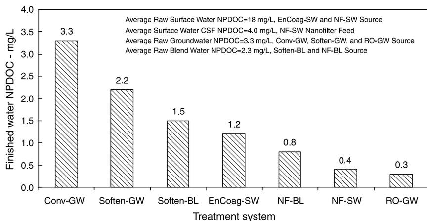
**Figure 3** | Finished water NPDOC by treatment system. RO = Reverse Osmosis, GW = Groundwater, NF = Nanofiltration, SW = Surface Water. EnCoag = Enhanced Coagulation, BL = Blend, Conv = Conventional Treatment, Soften = Softening, NPDOC = nonpurgeable dissolved organic carbon, CSF = Coagulation-Sedimentation-Filtration.
