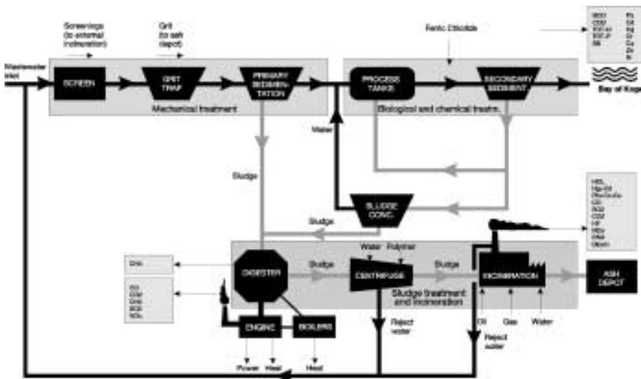
Figure 1 Avedore WWTP-Process, Consumption and Discharges/Emissions
