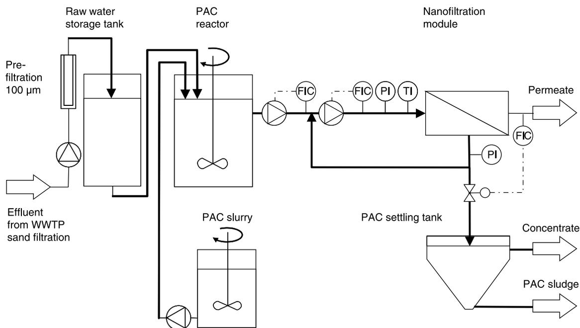
**Figure 1** | Experimental set-up of the pilot plant.
