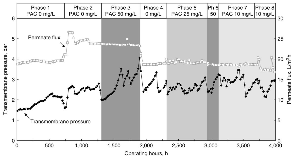
**Figure 2** | Phases and operational characteristics of the PAC-NF pilot plant tests (daily averages of online measurements).
