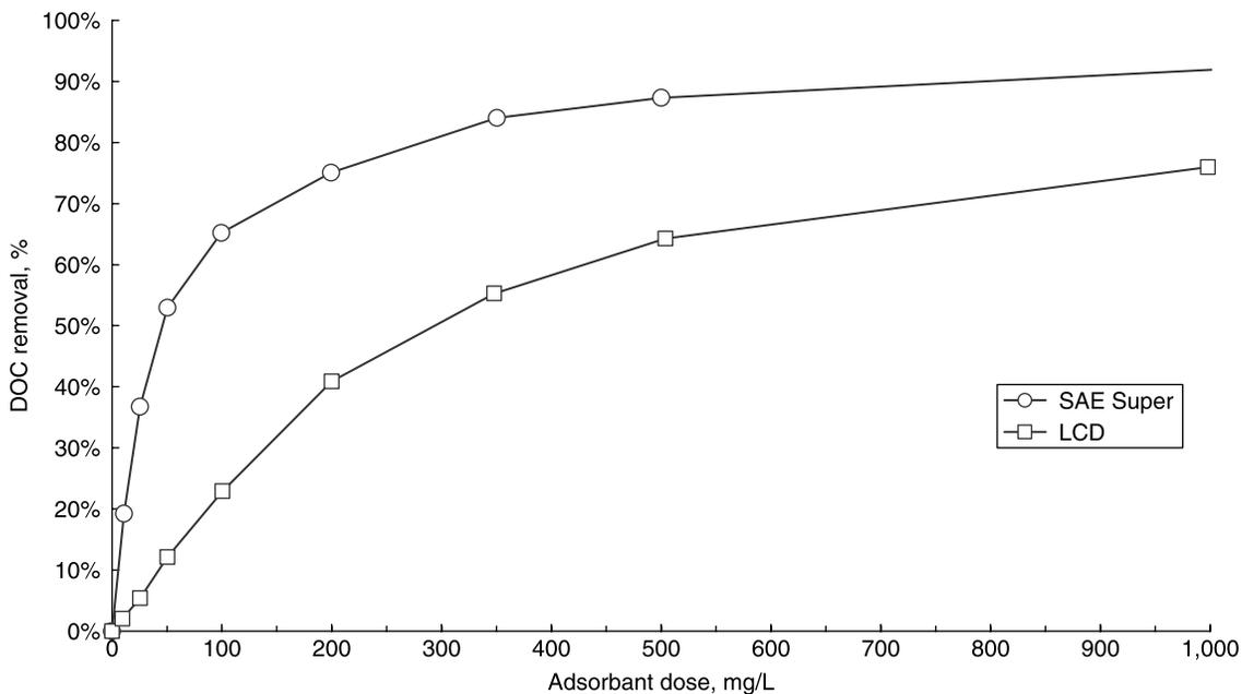
Figure 5 | Batch adsorption tests: DOC adsorption vs. adsorbent dose ( $\text{DOC}_0 = 4.5 \text{ mg/L}$ ).
