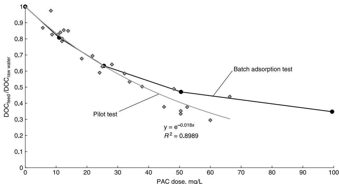
**Figure 8** | Comparison of DOC adsorption in PAC-NF pilot test and batch test (regression equation for pilot test).
