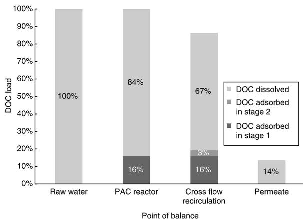
Figure 7 | PAC-NF pilot tests: DOC mass balance (PAC dose 10 mg/L).
