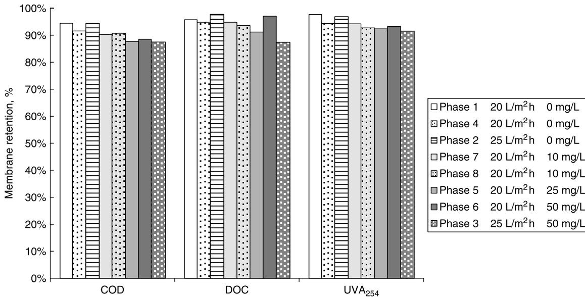
Figure 4 | PAC-NF pilot tests: membrane retention of organic substances ( $R_{\text{membrane}} = 1 - C_{\text{permeate}}/C_{\text{concentrate}}$ ).
