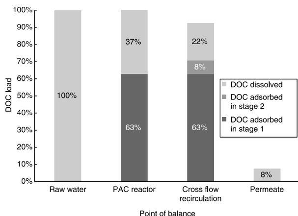
Figure 6 | PAC-NF pilot tests: DOC mass balance (PAC dose 50 mg/L).
