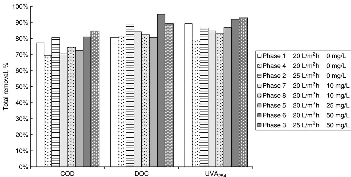
**Figure 3** | PAC-NF- pilot plant Soers: Total removal of organic substances ( $R_{\text{plant}} = 1 - C_{\text{permeate}}/C_{\text{raw water}}$ ).
