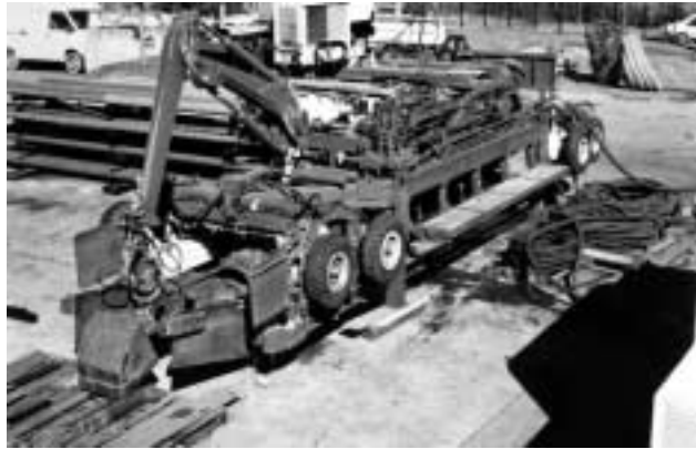
Figure 1 Mechanised flushing machine, referred to as CIRCE
