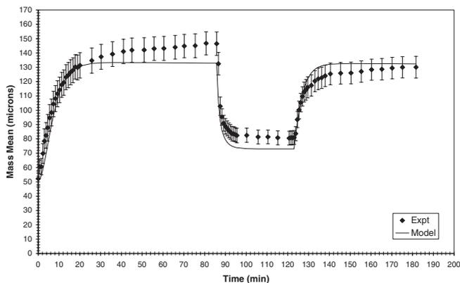
**Figure 3** Comparison between experimental and simulated results for step change in shear rate
