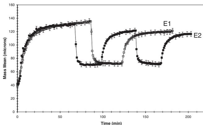
**Figure 1** Effect of step change in shear rate on floc size
