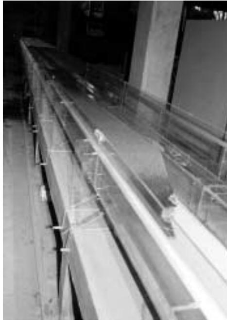
**Figure 4** Physical model of the BIEVRE interceptor
