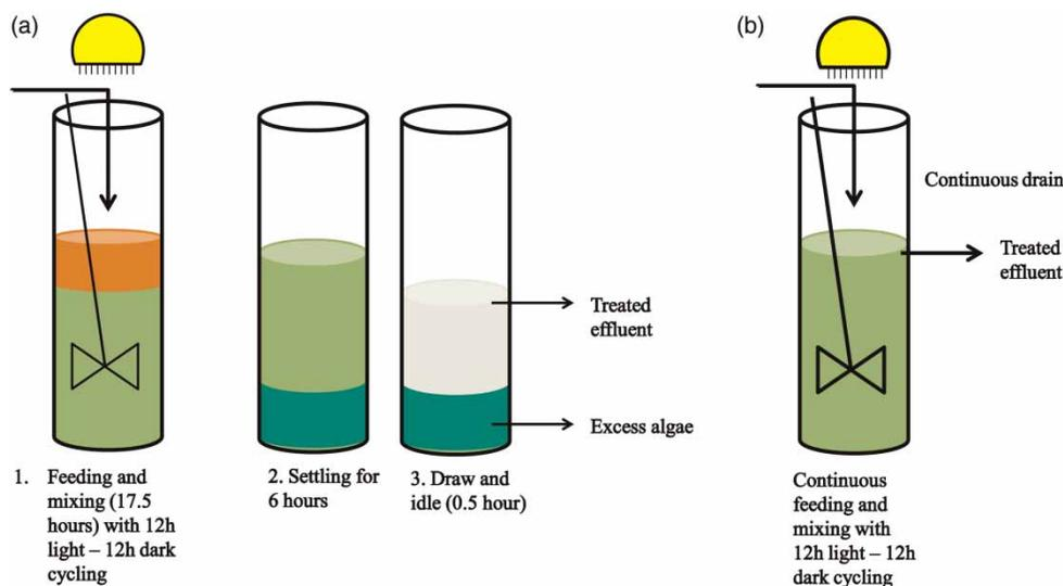
Figure 1 | Daily operations of reactors. (a) SBR. (b) CFR.
