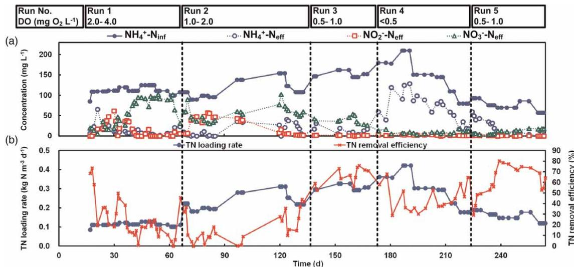
Figure 2 | (a)  $\text{NH}_4^+\text{-N}$ ,  $\text{NO}_2^-\text{-N}$  and  $\text{NO}_3^-\text{-N}$  concentrations; (b) TN loading rate, TN removal rate and TN removal efficiency of continuous-flow hybrid biofilm-carrier reactor.
