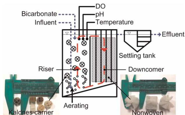
Figure 1 | Schematic diagram of hybrid biofilm-carrier reactor.
